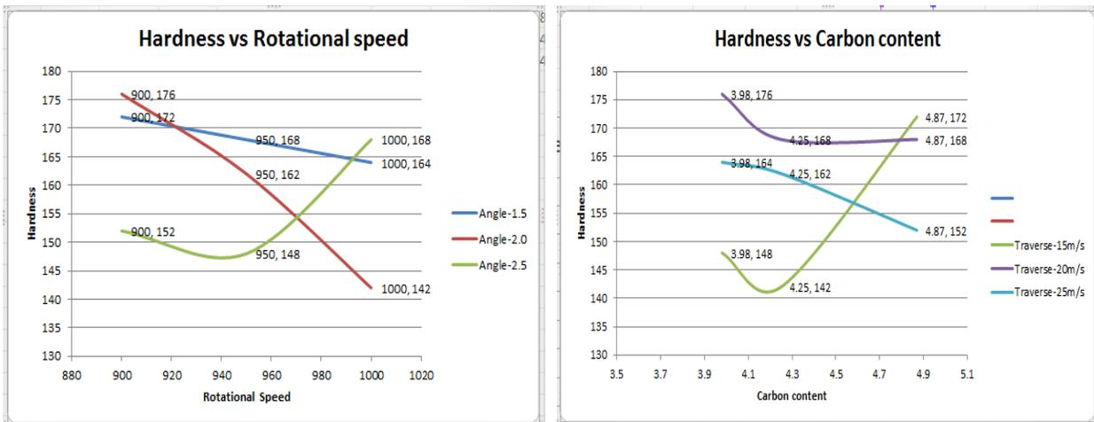
Figure.4: Hardness vs Rotational speed and Hardness vs carbon content
